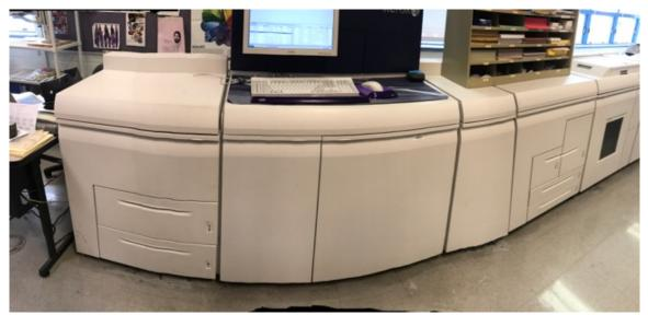
Name of the High Speed Black Production Printing press that has the (Feeder 1 module) with 2 paper trays, (Inserter A module) with 4 paper trays, A Basic Finishing Module, A Tape Binder Module and a Plockmatic Pro 30 connected to the end.
