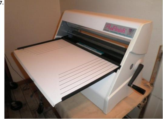
Device used to apply a 3 millimeter clear plastic film on to paper up to 24 inches wide.
