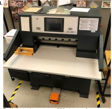
Device used to cut over 500 sheets of paper as long as 26 inches in width
